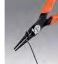
Round nose pliers are used mostly for bending and shaping wire.
