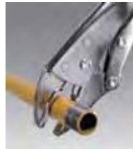
Gripping and welding pliers are used for clamping work pieces during welding and assembly work.
