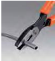
Combination pliers are used both for holding and for cutting.
