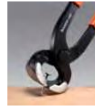
Pincers are mainly intended for pulling nails, but can also be used for medium hard wire.
