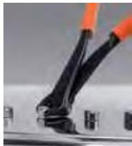
Nut pliers are intended to use for gripping small nuts (counter grip) in confined spaces.
