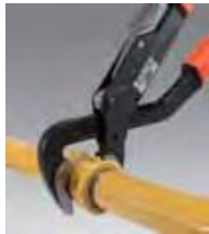
Slip joint pliers have an adjustable joint which provides a wide range of jaw openings and a firm grip on work pieces of varying shape.
